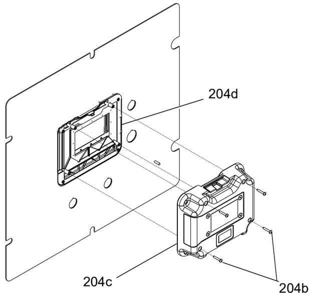
6. Remove rear display panel (204c) and disconnect display cable and key switch cable (239) from circuit board.
