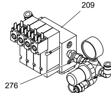
6. Repair or replace alternator regulator parts as necessary. See **Alternator Assembly**, page 84, for repair parts. Replace air regulator swivel fitting (276).
