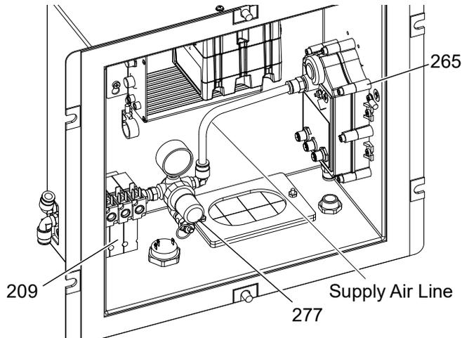
5. Loosen air regulator swivel fitting (276) and remove from solenoid module (209).
