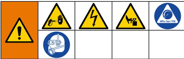
To avoid injury due to unexpected machine operation initiated by a remote controller, disconnect the customer I/O cable from the system prior to repair.
