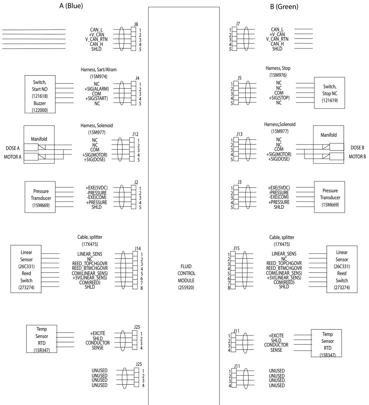
**NOTE:** NC indicates the wire is not connected.
