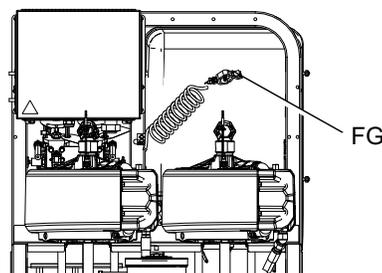
**Air and fluid hoses:** Use only electrically conductive hoses with a maximum of 500 ft (152 m) combined hose length to ensure grounding continuity. Check electrical resistance of hose regularly. If total resistance to ground exceeds 29 megaohms, replace hose immediately.
