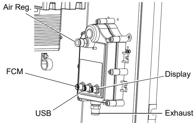
6. Disconnect air regulator air line and exhaust air line.
