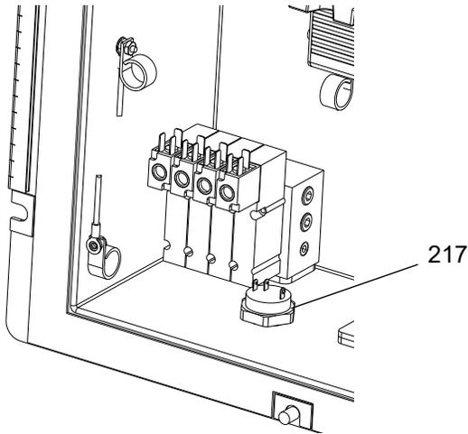
6. Screw in new alarm. Reconnect alarm wires. Refer to **Parts**, page 59.
