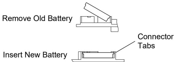
3. Replace with new battery. Ensure battery fits under connector tabs before snapping other end in place.
