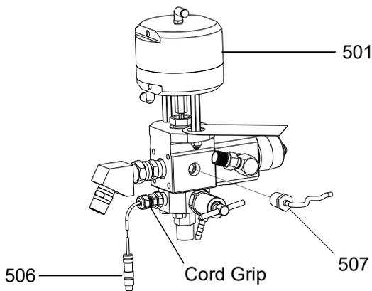
6. Replace with new fluid pressure sensor, and reconnect pressure sensor to FCM.
