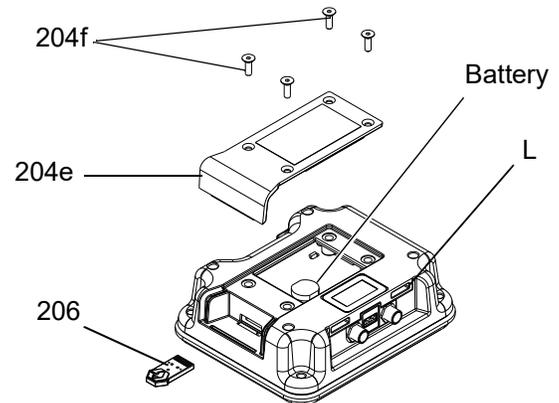
5. Insert and press token (206) firmly into slot.
