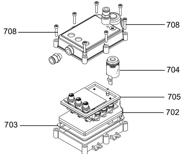
10. Replace gasket (702) and/or circuit board assembly (705) if damaged.
