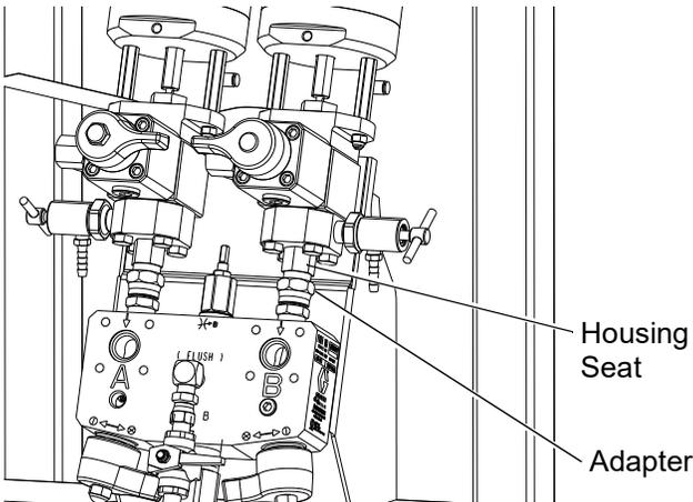
5. Disconnect RTD (506) from cord grip. Disconnect pressure sensor (507) and fluid line adapter from each dosing valve (501).
