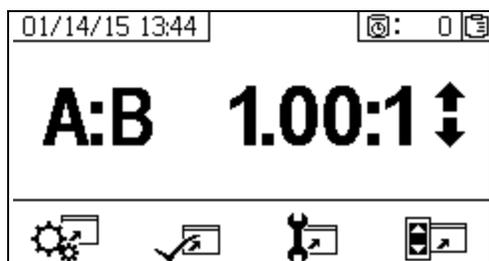
Home is the first screen that displays in Setup mode. It shows the current metering pump ratio and enables users to change the mix ratio and access the following screens: system setup, enable/disable functions, maintenance setup, and limits. Refer to the following table for more details.
