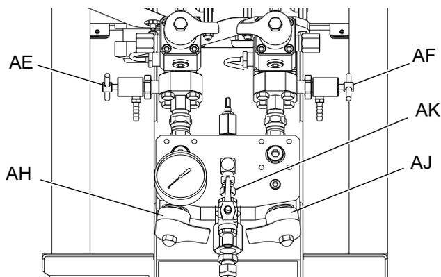
3. Open solvent shutoff valve (AK) at mix manifold.
