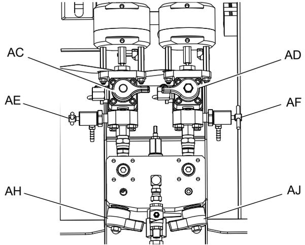
6. Place a clean container under sampling valve A (AE).
