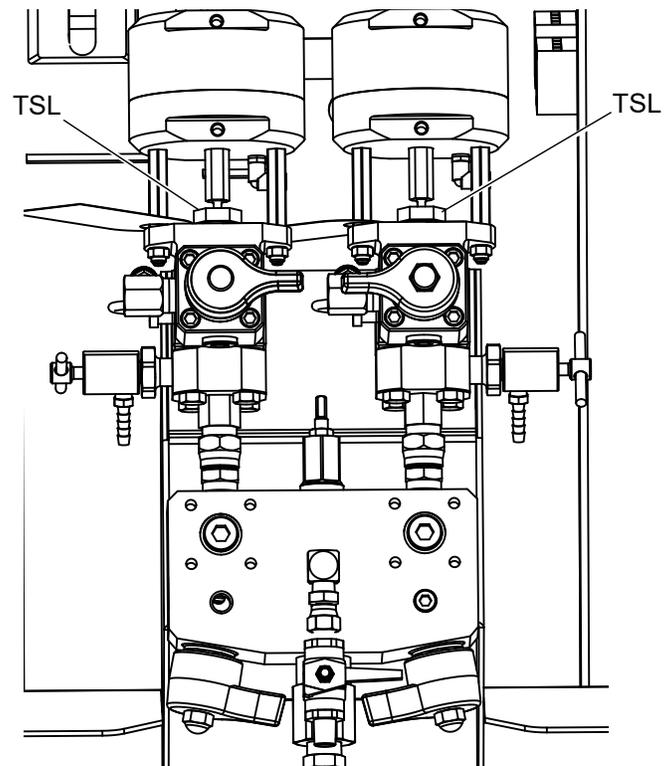
For pump and dosing valves, check packing nut tightness after first hour of operation and again after 24 hours. Then check when TSL discolors or seeps over packing nut. Also check tightness whenever sprayer is transported. Tighten packing nuts only when all fluid pressure is relieved. Continue to follow maintenance procedure intervals regarding all seals, page 64.
