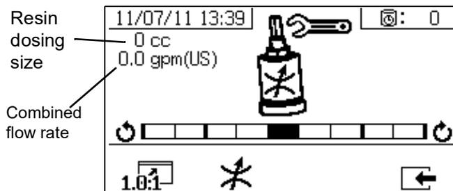
The restrictor adjust bar graph is shown when **\*** is pressed. This screen is used to adjust the restrictor.
