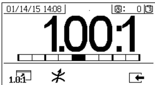
The ratio bar graph is shown when **1.0:1** is pressed. This screen is used to show the accuracy of the spray ratio. The bar should be in the center three segments when the restrictor is adjusted.
