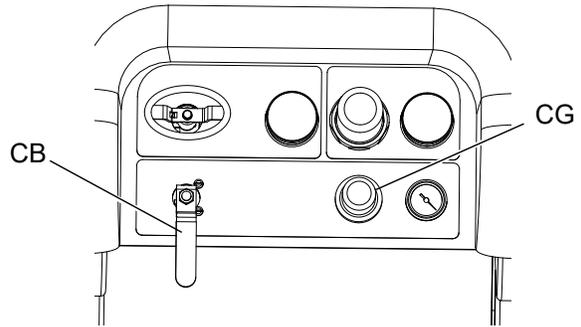
7. Close solvent pump air valve (CB) and trigger gun to relieve pressure. Engage gun trigger lock.
