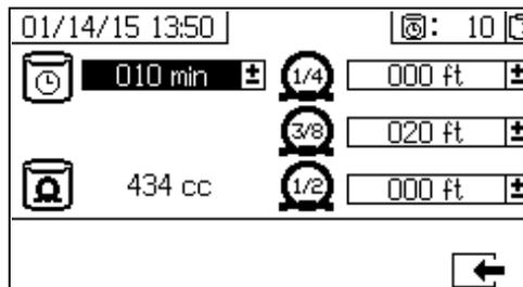
This screen enables users to set the potlife timer, and length of each mixed material hose specific to the system. The total mixed material volume is then calculated and displayed on the page. The potlife time displays in the upper right corner.
