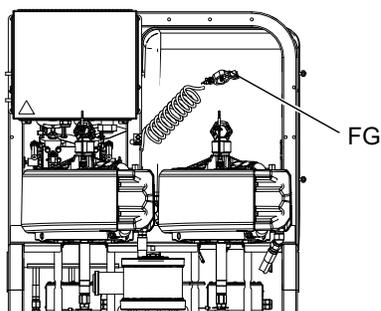
**Air and fluid hoses:** Use only electrically conductive hoses with a maximum of 500 ft (152 m) combined hose length to ensure grounding continuity. Check electrical resistance of hose regularly. If total resistance to ground exceeds 29 megaohms, replace hose immediately.
