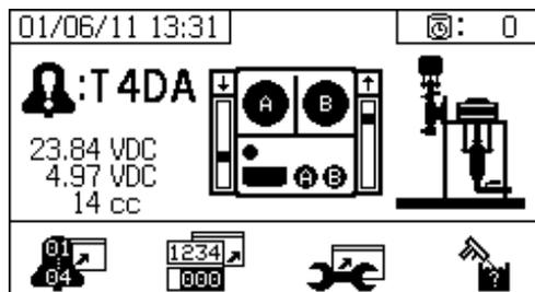
There are two levels of error codes: alarms and advisories. A bell icon indicates an alarm. A solid bell icon with an exclamation point and three audible alerts indicate a alarm. And an outlined hollow bell icon and a single audible alert indicate an advisory.
