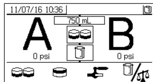
If the system ratio mode is by volume, either volumes or weights can be measured.
