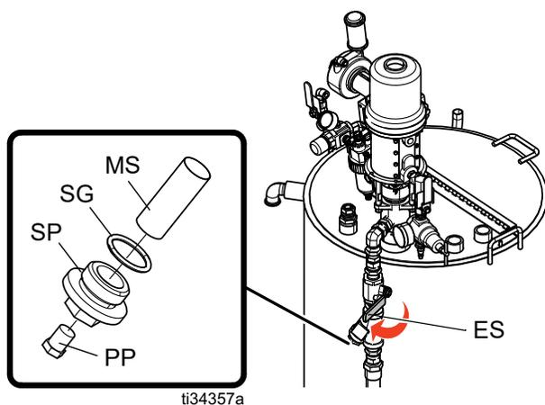
4. Inspect the screen. No more than 25% of the mesh should be restricted. If more than 25% of the mesh is blocked, replace the screen. Inspect the gasket and replace as needed. See your heated hopper manual for replacement components.
