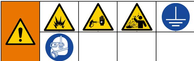
To avoid fire and explosion, always ground equipment and waste container. To avoid static sparking and injury from splashing, always flush at the lowest possible pressure.
