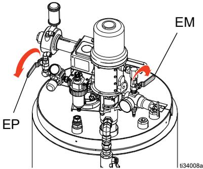
11. Run the main high pressure fluid pumps until the material has been emptied out of the system, press
