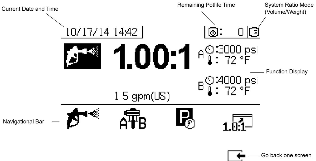
**FIG. 6: Main Display Screen Components (shown with all display features enabled)**
