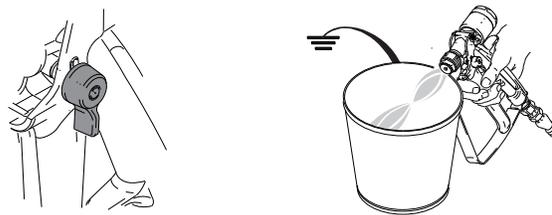
6. Close solvent pump air valve (CB).
