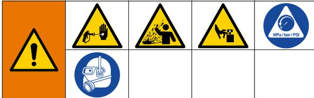
This equipment stays pressurized until pressure is manually relieved. To help prevent serious injury from pressurized fluid, such as skin injection, splashing fluid and moving parts, follow this Pressure Relief Procedure when you stop spraying and before cleaning, checking, or servicing the equipment.
