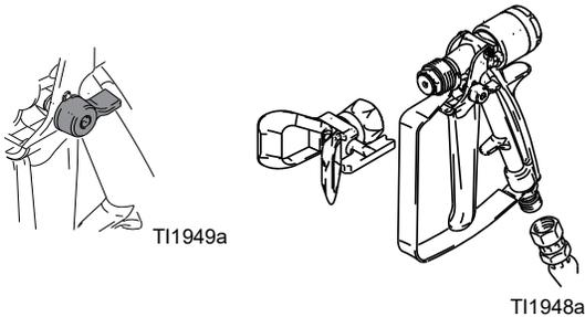
5. Disengage trigger lock and trigger gun into a grounded pail. Use a pail lid with a hole to dispense through. Seal around hole and gun with a rag to prevent splash back. Be careful to keep fingers away from front of gun.
