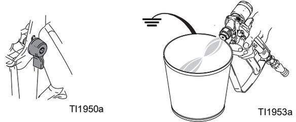
6. Open solvent pump air valve (CB). Pull out and slowly turn solvent pump air regulator (CG) clockwise to prime solvent pump and push air out of mix hose and gun. Trigger gun until all air is purged.
