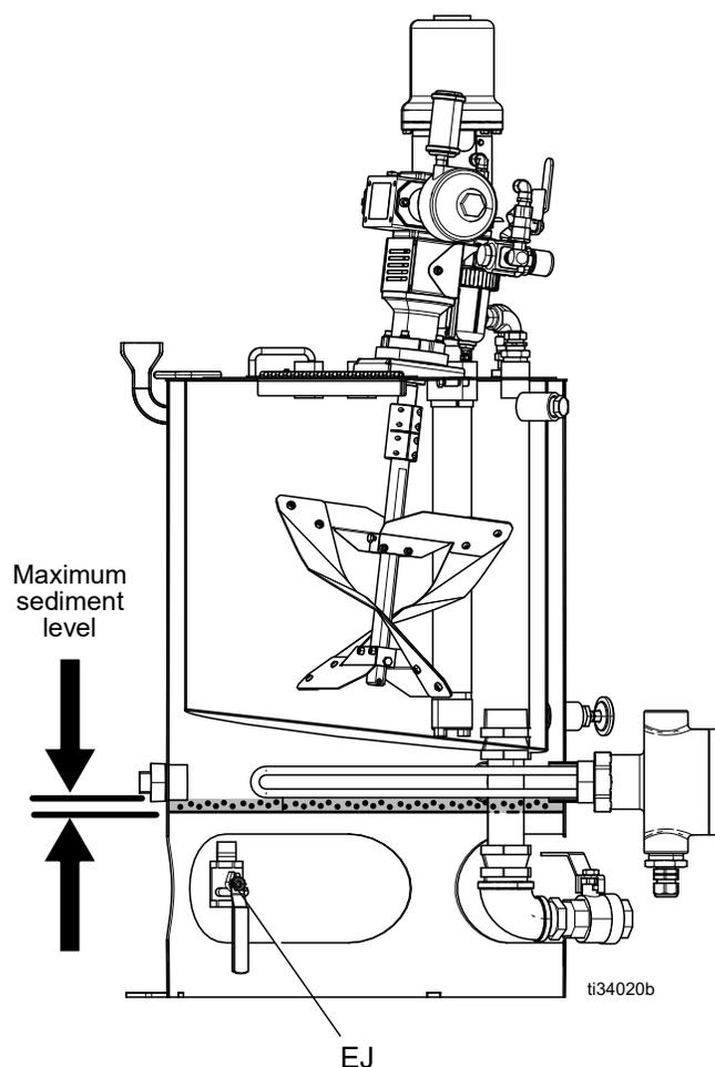
**NOTE:** The immersion heater will not operate in sediment deposits.
