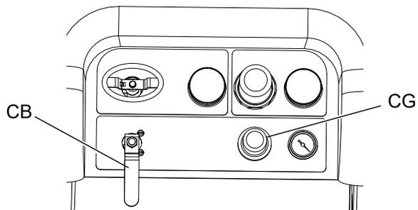
5. Disengage trigger lock. Hold a metal part of the gun firmly to a grounded metal pail with a splash guard in place. Use a pail lid with a hole in it to dispense through. Be careful to keep fingers away from the front of the gun. Trigger gun until clean solvent appears.
