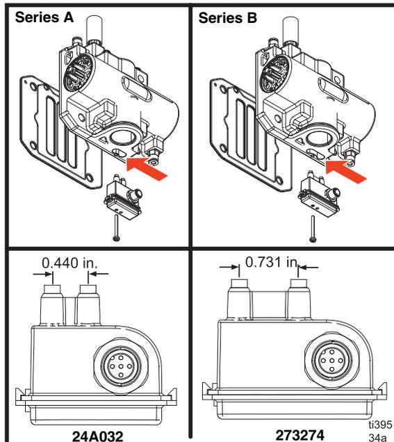
\* Series A air valves are needed for kits 24X550 and 24X552.
