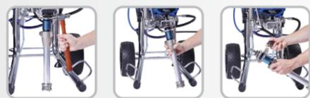
Loosen the Clamping Nut
