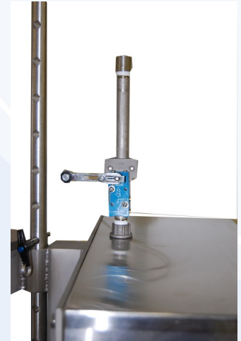
Low Level Control
