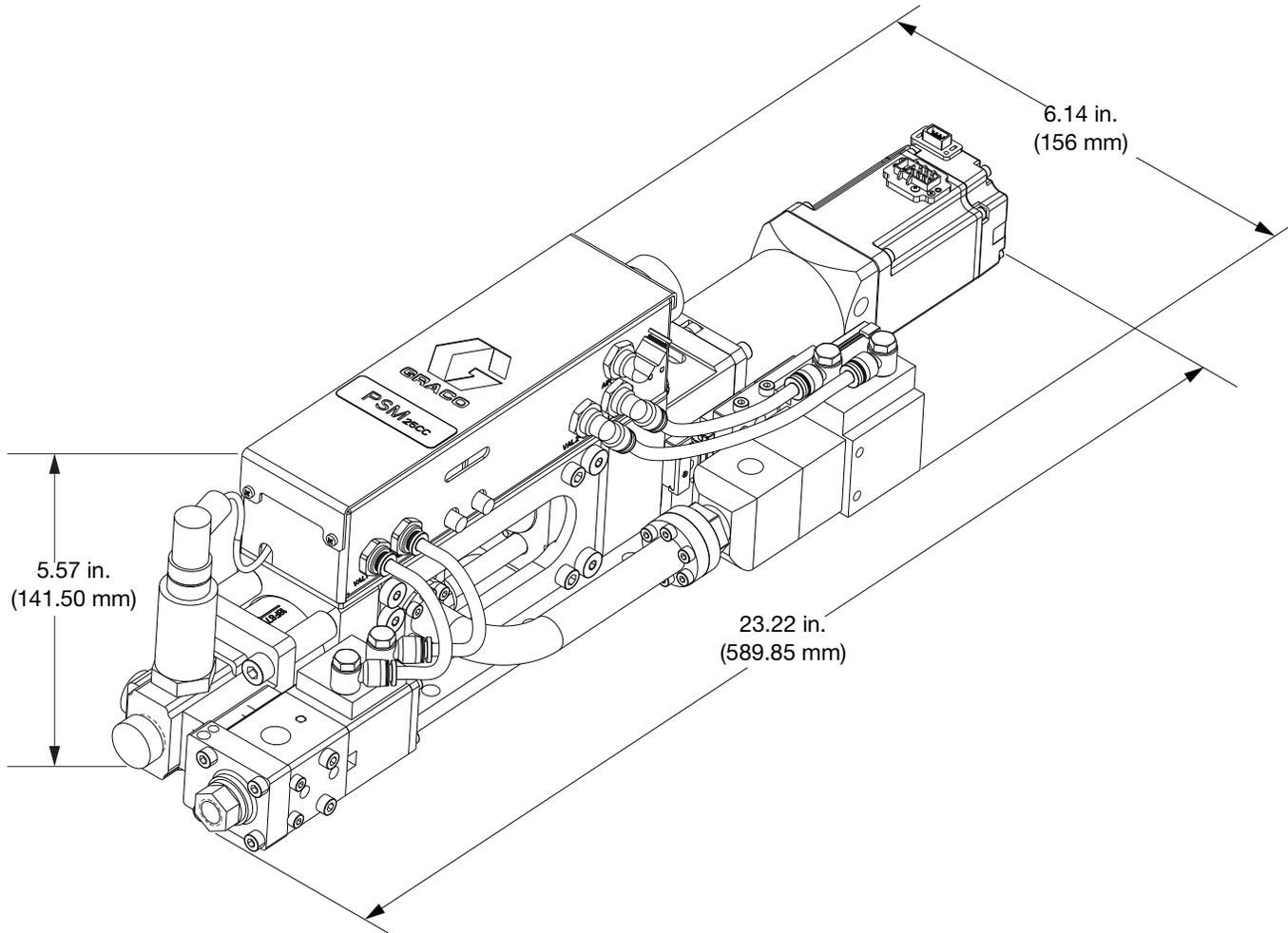
**FIG. 37: PSM Machine Dimensions, 25 cc**
