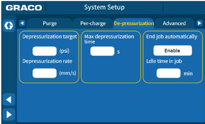
**FIG. 27 De-pressurization Setup Screen**
