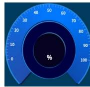
This displays how much material is in the cylinders (0-100%). When the rod slider is at the home position, 'Volume in cylinder' will show 100%. When the slider moves to the 'empty' position, 'Volume in cylinder' will show 0%.
