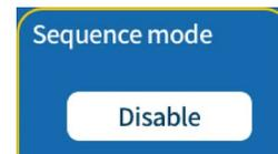
Press the button to enable or disable this function. The green color of the button indicates the sequence mode is enabled.
