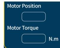
To Show the number of motor steps. The torque of the drive motor is shown in N•m.
