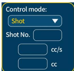
In Shot mode, the selected style number, target flow rate and target volume will be shown. Shot style can be selected by touch screen or customer signals. Preset styles include 40 styles, 0-39.
