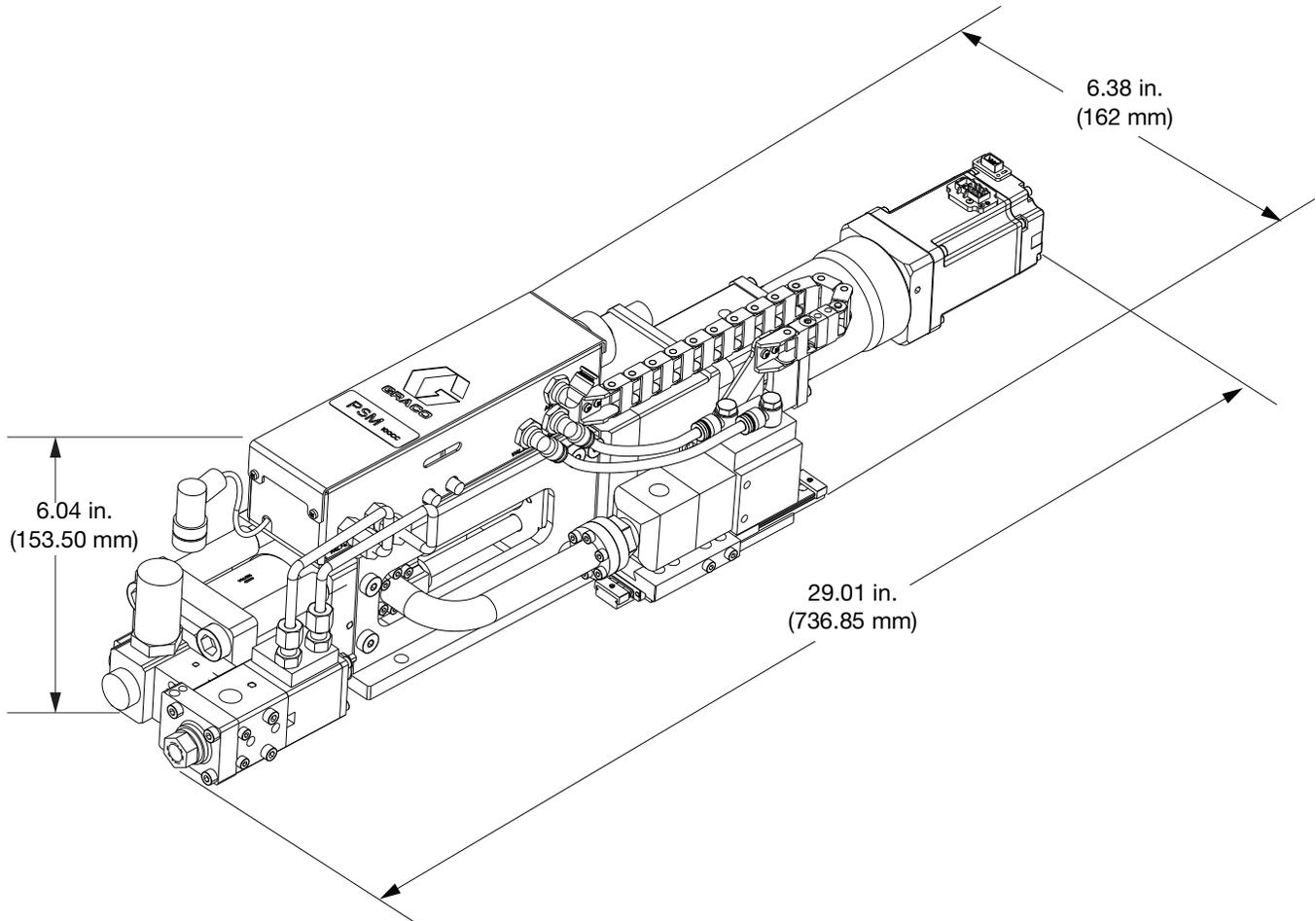
**FIG. 39: PSM Machine Dimensions, 100 cc**
