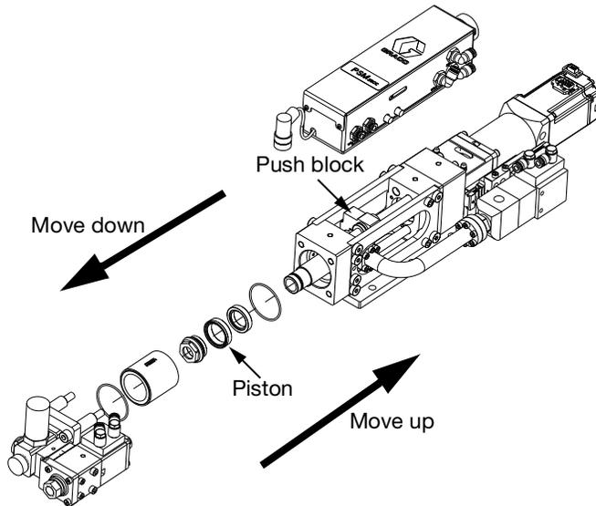
FIG. 32 Piston move up or down
