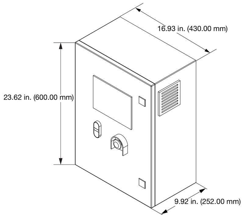
**FIG. 40: Control Box Dimensions**
