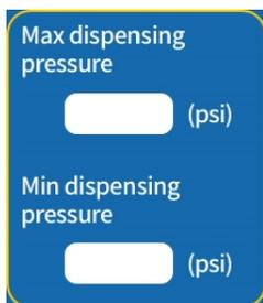
If the pressure is higher than the preset max pressure, the system will activate the alarm and send the alarm signal to customer system.
