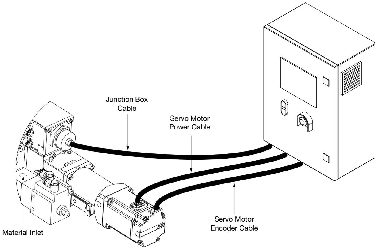
**Fig. 9: Cable Connections - Supply Pump Feed Version**
