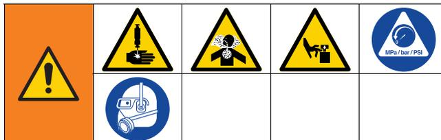
This equipment stays pressurized until pressure is manually relieved. To help prevent serious injury from pressurized fluid, such as skin injection, splashing fluid and moving parts, follow **Pressure Relief Procedure**.
