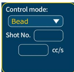
In Bead mode with preset value, the selected style number and target flow rate will be shown. The process for style number selection is the same as Shot mode.
