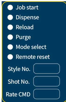
The input signals display shows the current signal status from customer inputs.
