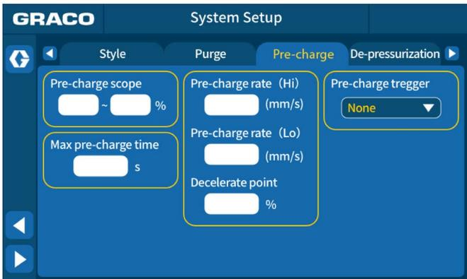
FIG. 26 Pre-charge Setup Screen
