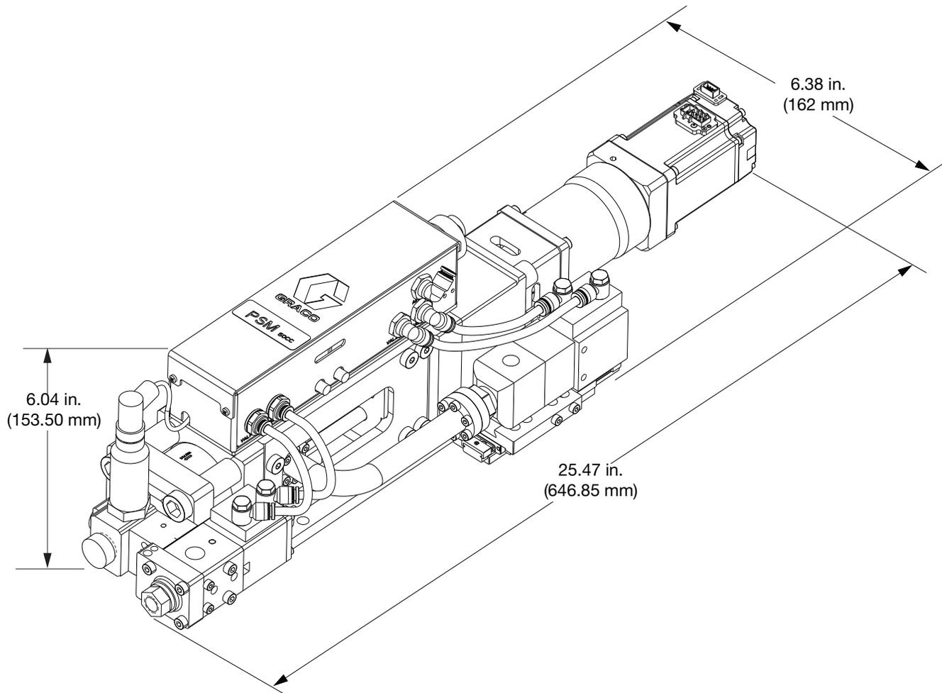
FIG. 38: PSM Machine Dimensions, 50 cc
