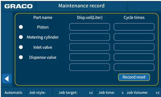
**FIG. 13 Automatic Screen 4 - Maintenance record**
