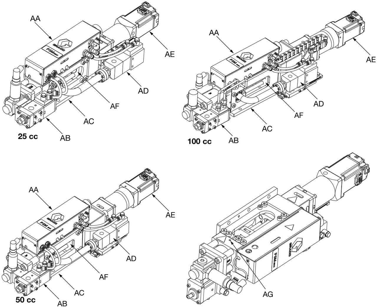
**FIG. 2: PSM Machine, Supply Pump Feed**
