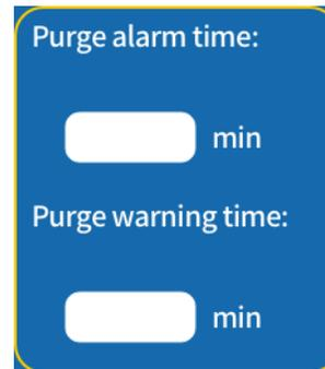
Set the purge request time. When the equipment doesn't dispense, the PSM control box will start the countdown for the time chosen by the operator. When time is up, the system will send out the purge alarm signal and show 'purge request' in the information bar.
