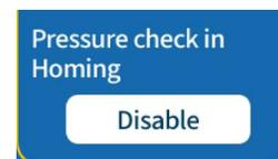
Press the button to enable or disable this function. The green color of the button indicates pressure check after homing is enabled.
