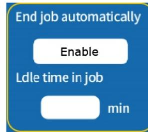
After this option is enabled, the operator must set the maximum idle time for the system while performing a job. After the set period passes without any operation, the depressurization program will be automatically executed and the current job ended.
