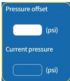
The operator may input values to adjust the pressure offset on the sensors.
