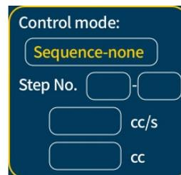
In Sequence mode, the step number, remaining repeat times, target flow rate and volume will be shown in different screens based on different step types. The operator can edit the step by using the touch screen prior to or following the current job. Once dispensing has begun, the 'Control mode' display will show the current step, including sequence shot, sequence bead sequence reload and sequence none.
