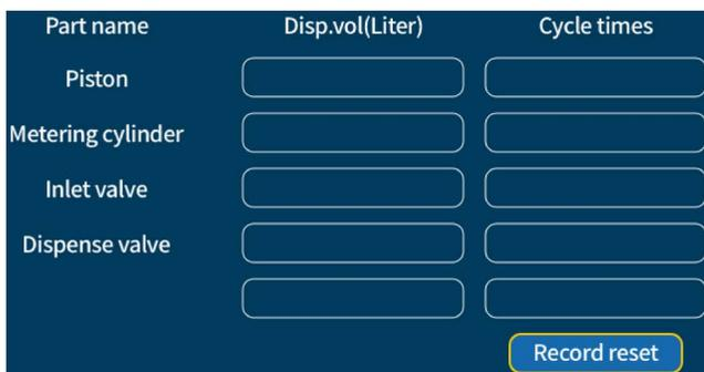
To record the workload of important parts. Click the 'Record reset' button to reset the data. The last section box records the statistics workload. This data cannot be reset.
