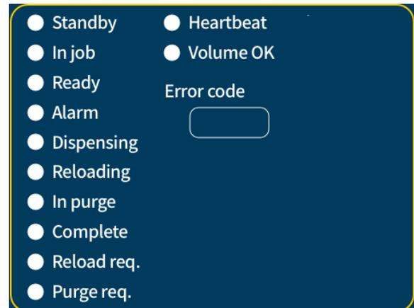
The output signals display shows the current signal status from the PSM control box.
