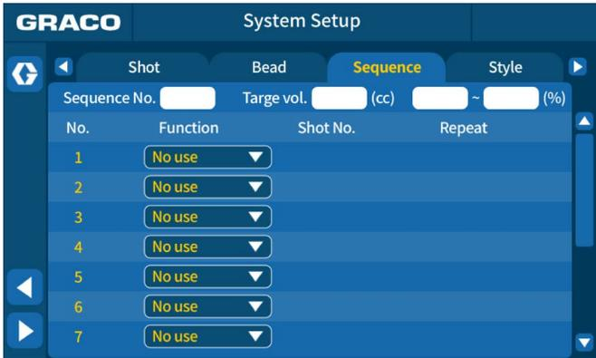
**FIG. 23 Sequence Setup Screen**
