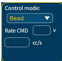
In Bead mode with custom setting, 'Rate CMD' will be shown as voltage value and target flow rate will be shown. The flow rate will change based on rate command.
