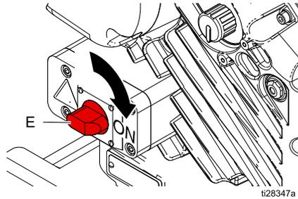
10. To start pump, pull out pressure adjustment knob (H) and turn clockwise slowly to increase pressure, until a steady stream flows from drain valve. Push knob in to lock.
