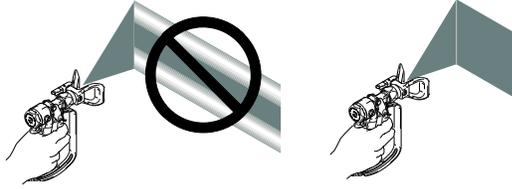
**NOTE:** When determining the desired spray pressure, always increase the spray pressure until the spray pattern fully develops. This will reduce the pressure surge when the pump is stalled and minimize over-spray.
