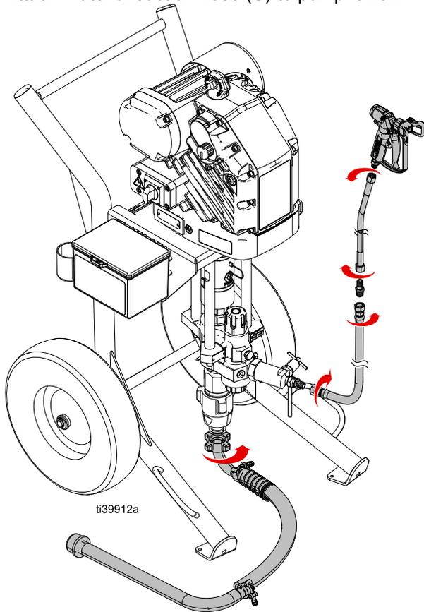
**NOTE:** Maximum suggested length is 6 ft (1.8 m), minimum suggested inner diameter is 1 in. (2.5 cm).
