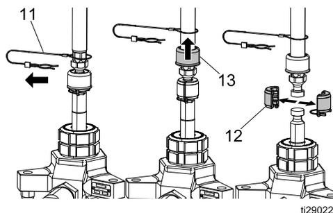
7. Use a wrench to hold the tie rod flats to keep rods (8) from turning. Unscrew nuts (10) and remove the lower (9).
