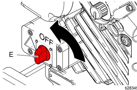
4. Disengage gun trigger lock.
