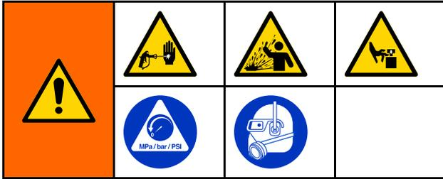
This equipment stays pressurized until pressure is manually relieved. To help prevent serious injury from pressurized fluid, such as skin injection, splashing fluid and moving parts, follow the Pressure Relief Procedure when you stop spraying and before cleaning, checking, or servicing the equipment.
