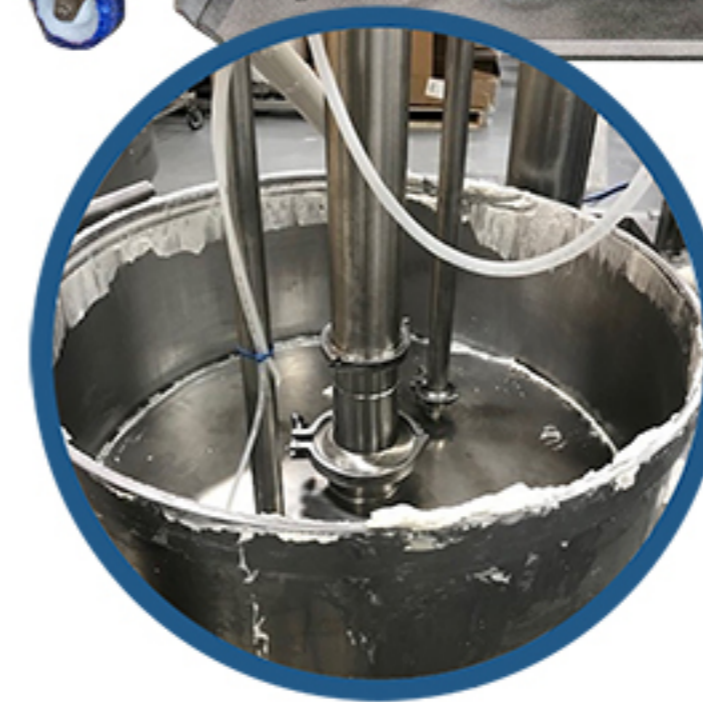
Ram in action pumping frosting out of a Topos Mondial mixer bowl
